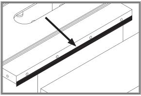
**Figure 15.** Masking tape location for shimming the wing up.
